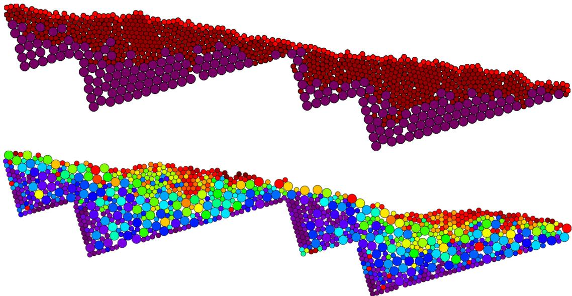
Fig. 1. Distribution of particles on a moving grate at the initial time  $t=0$  s (above) and the final time  $t=600$  s (below). For brevity, only the particles are shown, but not other structural elements. Particles of different temperatures are shown in different colors.
