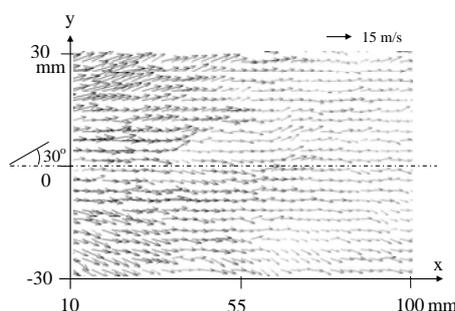
Fig. 2 Velocity vectors at an instant time in flow field for Type D60c ( $Re=8,400$ ).
