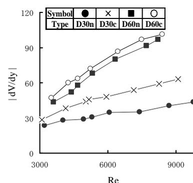
Fig. 3 Change of the jet-stream velocity-variation rate,  $|dV/dy|$  versus Reynolds number.
