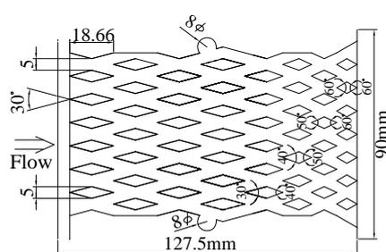
Fig. 1 Schematic diagram of the top view of the streamwise diverging diamond-shaped bundle.
