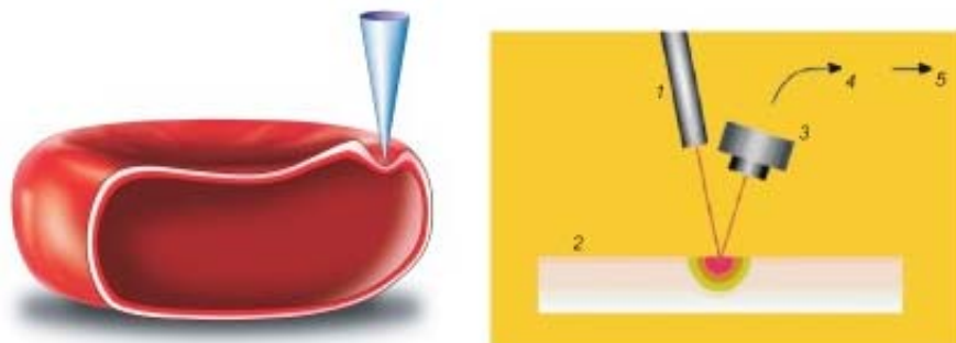
Fig. 1 Schematic illustration of AFM tip probing of single erythrocyte in-vitro (left) and laser inspection of erythrocytes motility in a living tissue in-vivo by DLS (right): 1 - laser; 2 - tissue under study; 3 - CCD camera; 4 - digital frame grabber; 5 - PC.
