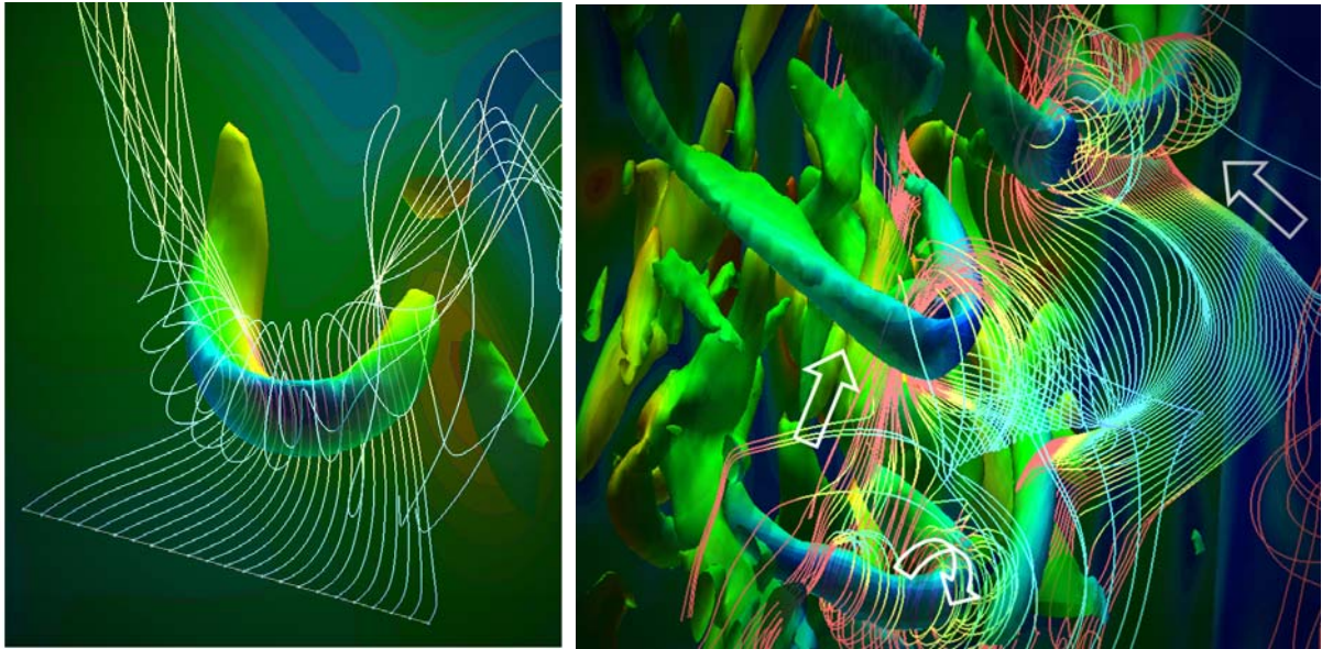
Fig. 9 Visualization of concentrated vortices developing in the BL by (left) t = 1.6 s and (right) t = 2.0 s. Isosurfaces of Q = 200 and 600 \text{ s}^{-2} colored by vertical velocity are shown for t = 1.6 and 2.0 s respectively
